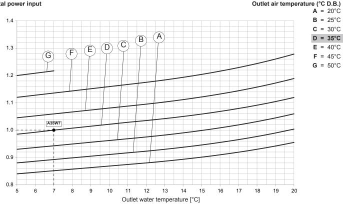
The standard performances refer to a 5°C temperature difference between the water entering and leaving the heat exchanger and to operation of the unit with all fans at nominal or maximum speed. A 0.44 x 10<sup>-4</sup> m<sup>2</sup> K/W fouling factor has also been considered with the unit installed at zero meters above sea level (Pb = 1013mbar).
